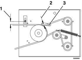
Figure 17 36 inch Belt Guide Location (Viewed from underneath the engine deck)
